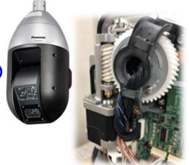
Around 4 times longer lifespan than conventional rubber belt drive
